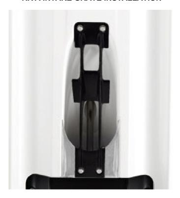
Install supplied RIVA intake plate using OEM bolts making sure front edge of ride plate is against hull and pump inlet shoe evenly.
