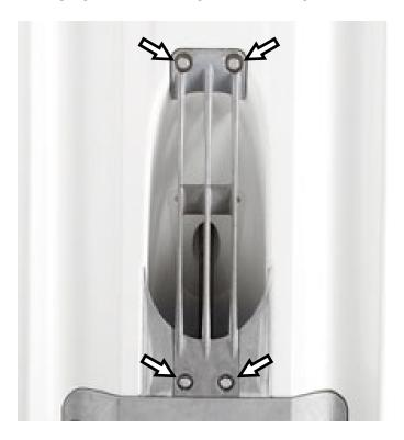
Remove OEM intake grate plate bolts (4). If necessary, use a heat gun to apply heat to bolt heads only!
