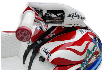
Hood Straps Installed
